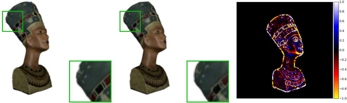
Figure 5: Visual comparison of two 200 \times 200 pixel views. Left: Full-resolution mesh (440,297 triangles, vertex colors). Center: Simplified 3D thumbnail with 256 \times 256 pixel texture (786 triangles). Right image: squared difference, multiplied by factor 8 for visualization purposes. Typical artifacts occur at the silhouette, due to reduced geometric fidelity, or at regions of fine texture detail, due to the small texture resolution.
